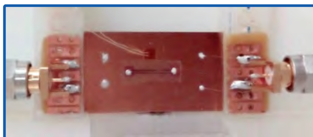
Figure 14 Experimental set-up for the simultaneous measurement of magneto-impedance, stress-impedance and MOKE hysteresis loop: Left: View of the actual sample-holder. Right: Scheme of the operation.
