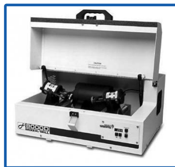
Figure 2 New equipment acquired during 2016: DIMATRIX DMVP-2831 2D ink printer for line of Materials for sensors (top left); SPEX SamplePrep 8000D Dual Mixer/Mill for mechanical alloying and nanomilling (top right); ONA prima E250, second hand spark cutter, for cutting and shaping metals and alloys (down).
